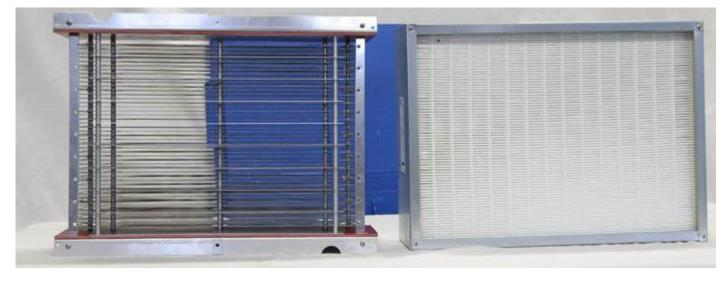
The photo above shows the Electrostatic filter along side of the HEPA filter we mentioned before. Note how much free air can pass through the Electrostatic vs the HEPA. The HEPA produces a 22% pressure drop where the Electrostatic only 4%.
