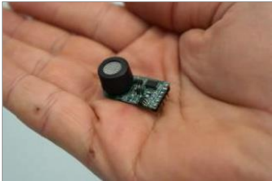
Figure 9. AR-5000 CO 2 sensor from PSS Korea
